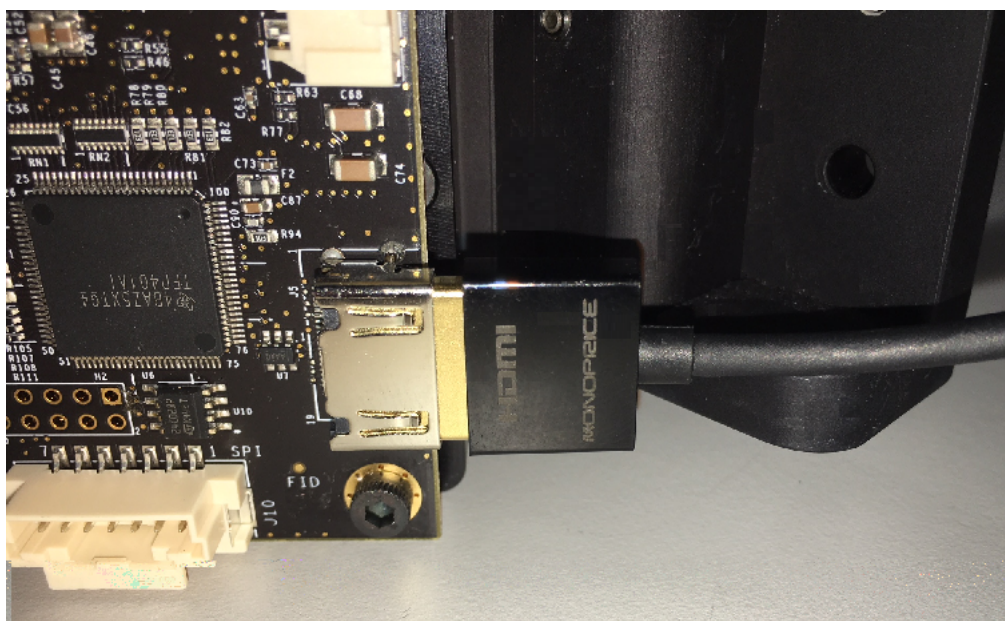
Figure 2-4. HDMI Cable Install
